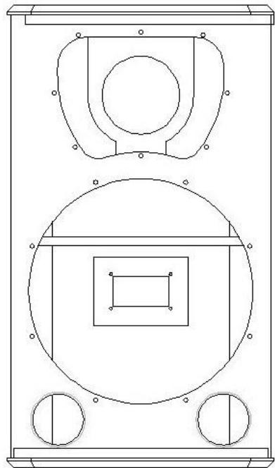
Equipped with one 15" speaker in a tuned enclosure. The HF section features one 2" compression driver from Celestion coupled to a rotatable diffuser, offering a dispersion of 90°x50° (H x V).
